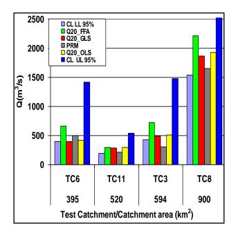
Figure 6.2.6 Comparison of flood quantiles for Q<sub>20</sub> (eastern NSW)
