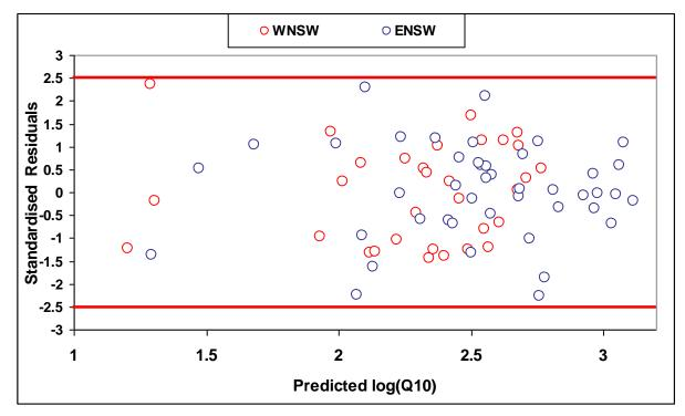
Figure 6.2.1 Standardised residuals vs predicted quantiles for ARI = 10 years (the red marks show the bound of  $\pm 2.5 \times \text{standardised residual}$ )
