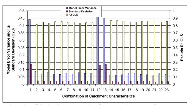
Figure 6.3.1 Selection of predictor variables for flood quantile model (ARI = 20 years)
