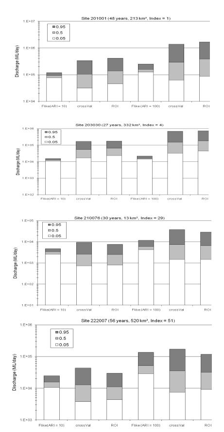
Figure 6.7.4 Posterior distribution of 10 and 100 years flood quantiles for four sites - 5, 50 and 95% posterior percentiles of the quantile are presented for the site data (labelled as FLIKE), fixed region GLS (labelled as crossVal) and ROI GLS (labelled as ROI)
