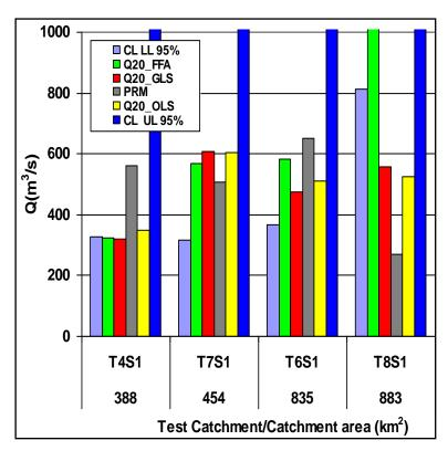
Figure 6.2.7 Comparison of flood quantiles for Q<sub>20</sub> (western NSW)
