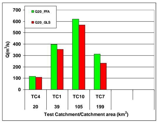
**Figure 6.2.8a** Comparison of flood quantiles for Q<sub>20</sub> (eastern NSW): QRT-GLS and at-site FFA estimates shown
