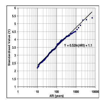
Figure 6.6.3 Frequency distribution of the standardised values (Y) and linear interpolating function
